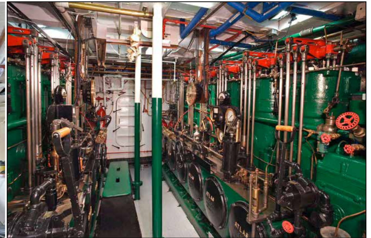
Entering the engine room is a true journey back in time. Dating from 1920, the two original Imperial Atlas diesel engines have been modernized to meet current safety standards.
